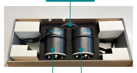
40 kHz DPC shear wave transducer
