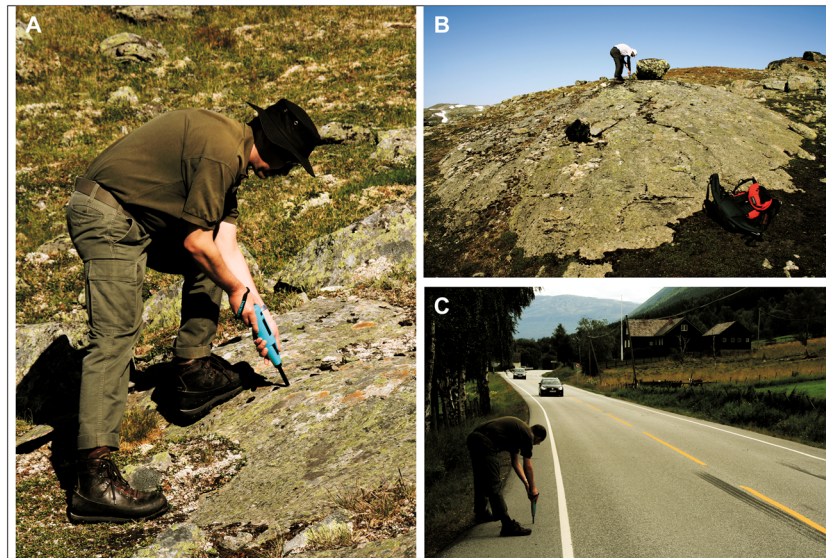
Figure 2. Field measurements with the SilverSchmidt (A) and the mechanical Schmidt hammer (B) at locality A (Leirbreen, outer site). (C) The tarmac test surface (see text). This figure is available in colour online at wileyonlinelibrary.com/journal/espl
